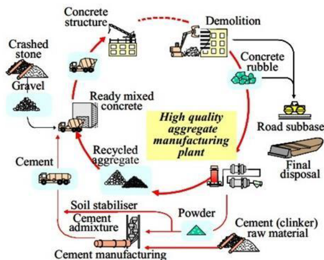
Figure 7. Supply chain of concrete waste recycling
